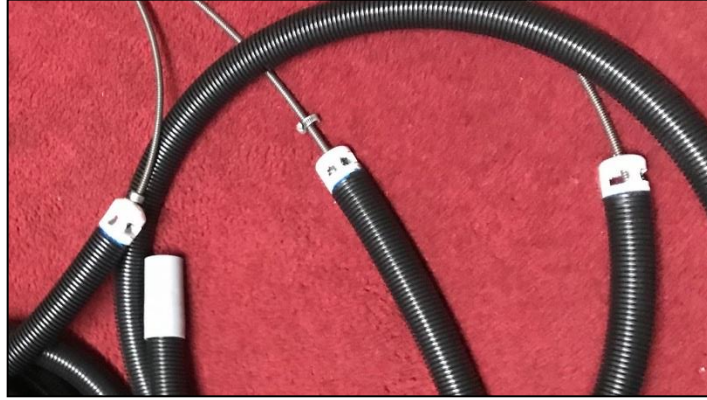
Figure 15—Final 1.25-in.-diameter hose configuration with plumber's snake.
