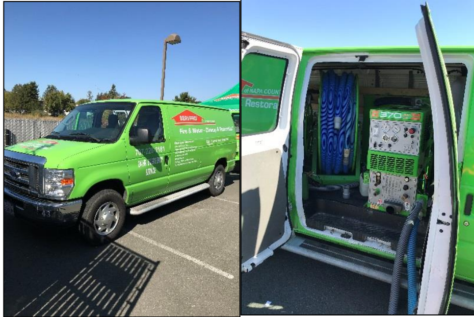
Figure 9 (left-right)—ServPro van and the interior showing vacuum hose and pumping system. Water storage tank (not pictured) is directly behind the pump.
