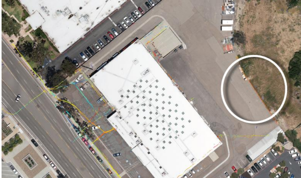
Figure 4—The map data in SubView shows multiple distinct utilities throughout the front and back parking lots. A line running along the canyon edge reveals a separate utility energized via signal bleed.
